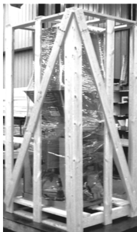
Figure 2-1. Typical Shell Crate
